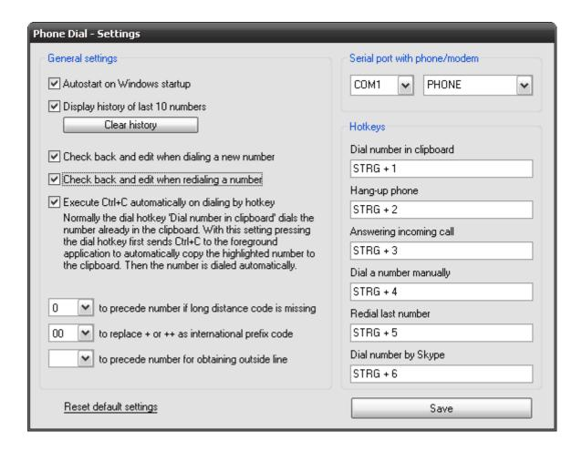
**Serial port with phone/modem:** The phone or modem with serial interface RS-232 is connected to the PC com port (COM1 to COM8). If a modem is connected for dialing then MODEM must be chosen.
