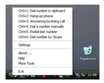
**Dial a number in clipboard:** Any phone number stated in any application (Word, Excel, Email, Browser etc.) can be highlighted with the mouse and then copied to the clipboard using the keyboard shortcut CTRL-C. Then, the number can automatically be dialed by using the individually defined hotkey (Standard CTRL+1).
